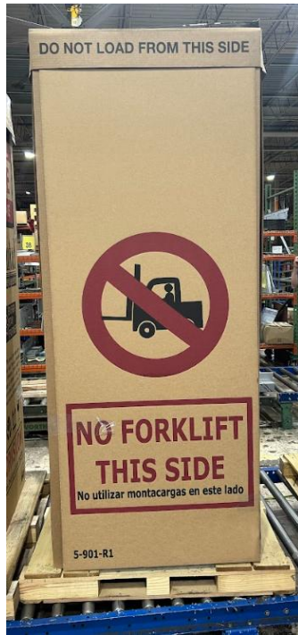
Figure 1. Example of manufacturer-applied handling instructions used to reinforce intended forklift entry direction and communicate handling requirements.
